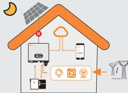
**Mode 3:** When grid fails, the system automatically switches to Back-Up mode. The Back-Up load can be supported by PV and battery.
